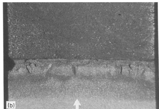
Figure 5 Fractographs of a (a) typical compression-compression fatigue precrack and (b) a precrack after compression fatigue followed by tensile fatigue. The arrows indicate the end of the precrack.
